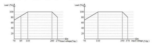
Input voltage and load characteristic curve
